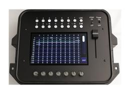
So now when I tap on 19, the red line disappears and there is a white line starting from address 19 covering the 12 channels from the Skypanel in mode 1.
