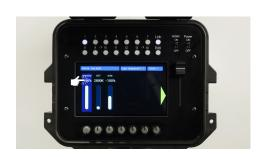
Push a fixture button to select the fixture you want to control. The display will show all the available faders for the selected fixture.
