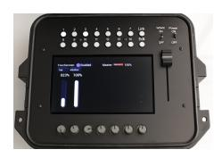
The MASTERFADER only controls the INTENSITY channels from the fixtures. Standard the option button is on ALL, at this point the MASTER controls all the patched fixtures.
