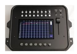
By selecting PATCH in the top left corner, the patch list opens and now I see that addresses 1 till 12 are underlined in red. This means there is a double patch on these addresses.
